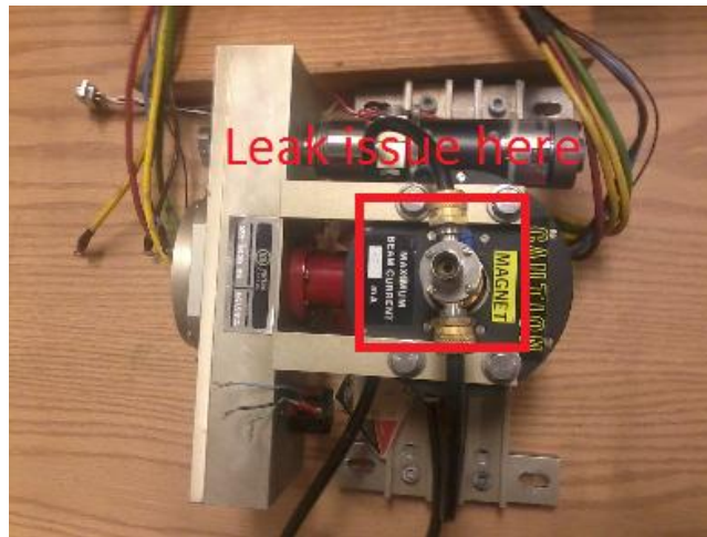
EO199C0 Leak Issue
