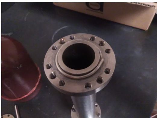
Figure 3: Inner Column with Indium Seal
