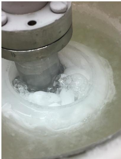
FIG. 7. Dry Ice and ethanol frozen solid due to surrounding liquid nitrogen
