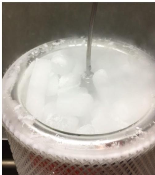
FIG. 8. Dry Ice and ethanol bath setup
