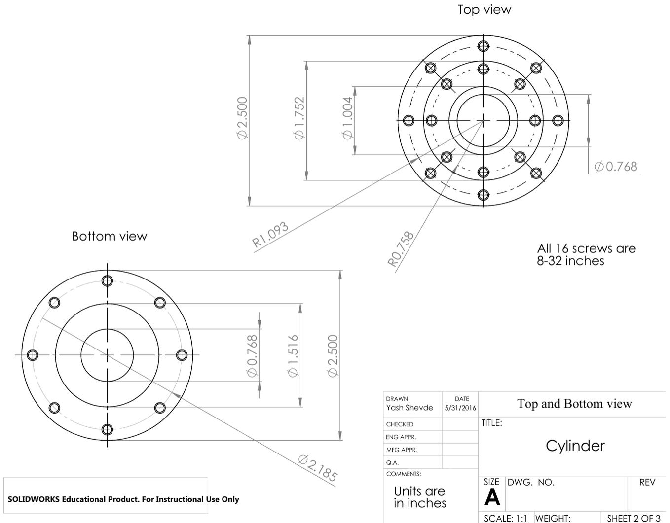
FIG. 15. The drawing of the cylinder end cap for solid ammonia making.
