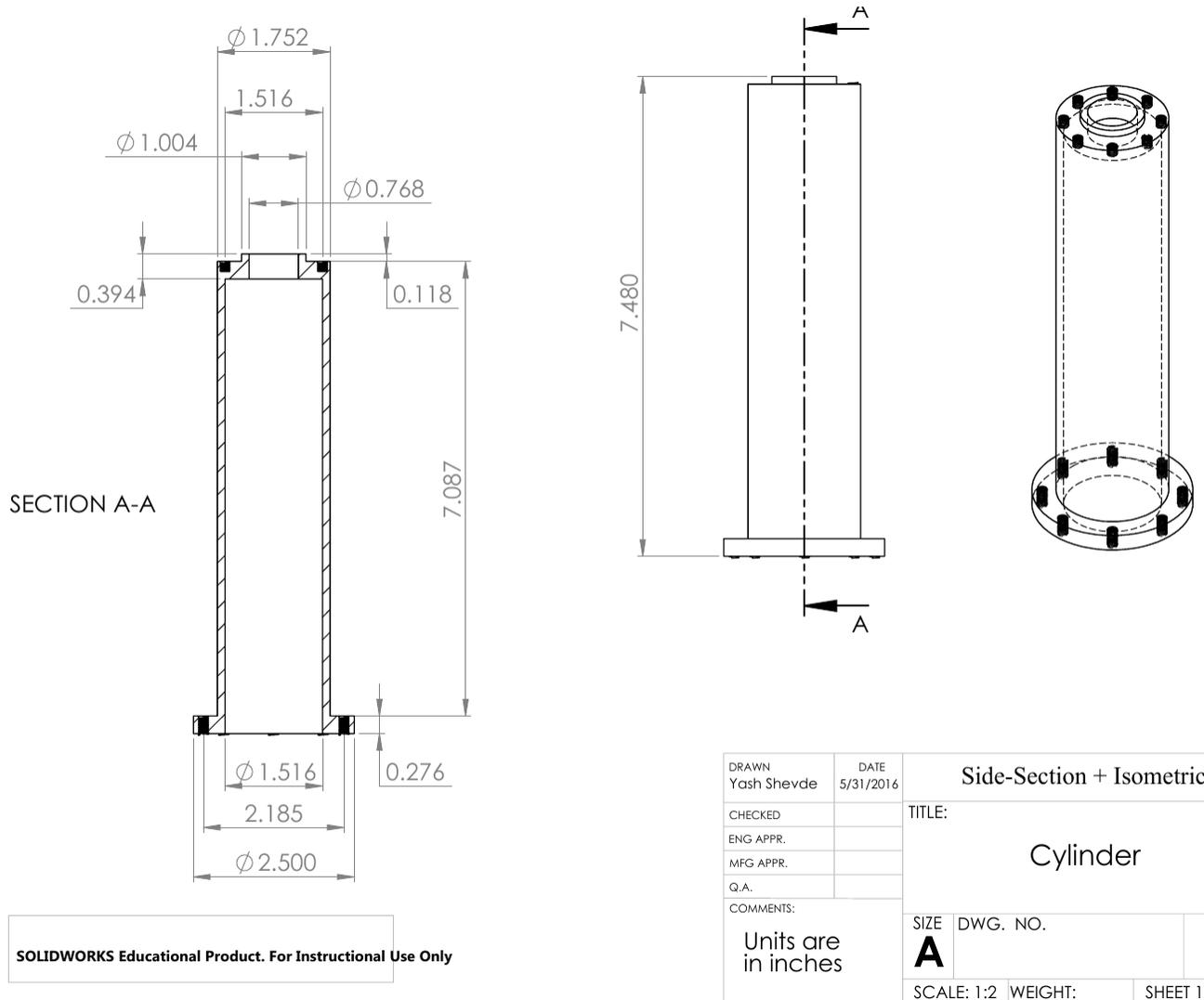
FIG. 14. The drawing of the cylinder for solid ammonia making.
