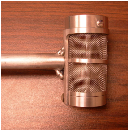
Figure 4.4: Irradiation basket used during target material irradiation at NIST.
