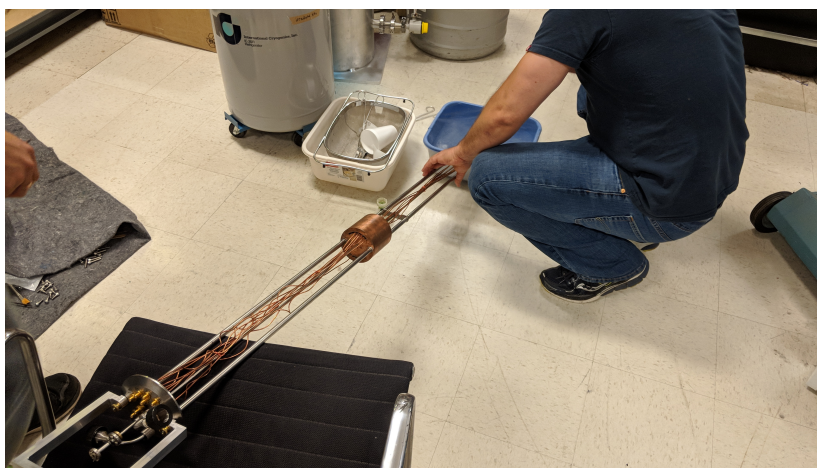
Figure 6: Place the target insert cup end into the liquid nitrogen at an angle for loading and unloading the target cups with the \text{NH}_3 beads.
