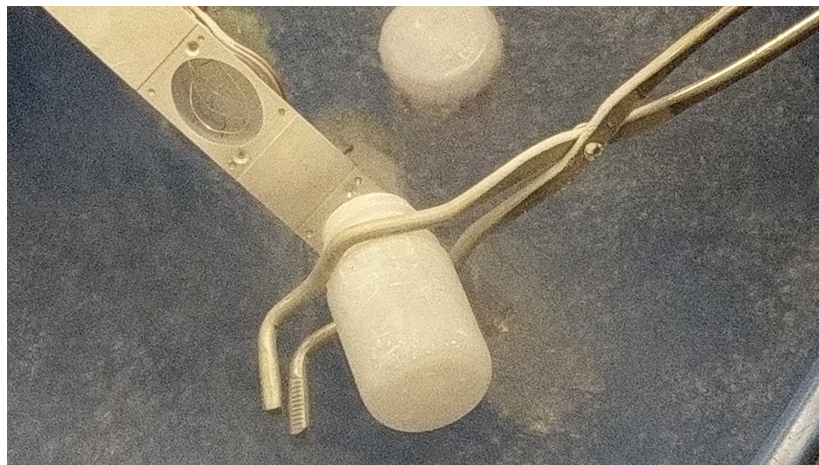
Figure 7: To fill the target cup carefully pour the target beads into the cell opening on the target insert, lifting the material out of the liquid nitrogen only for a few seconds at a time. Be careful not to lose material in the transfer process or to let the beads warm up.
