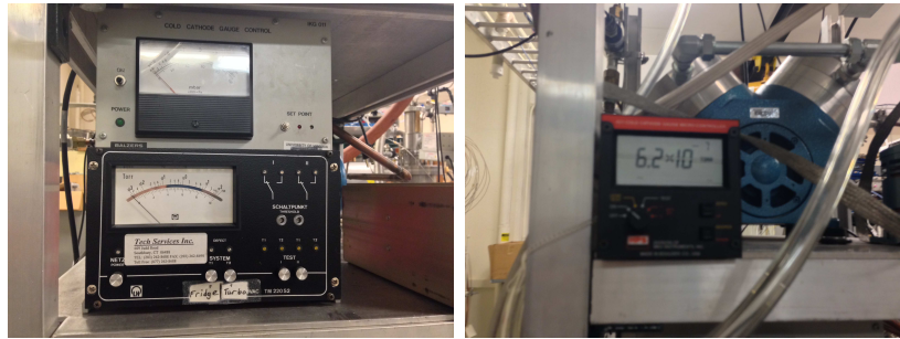
Figure 2: Electric pump (left) and The Pfeiffer Turbo pump (right) used to pump out the OVC/IVC.
