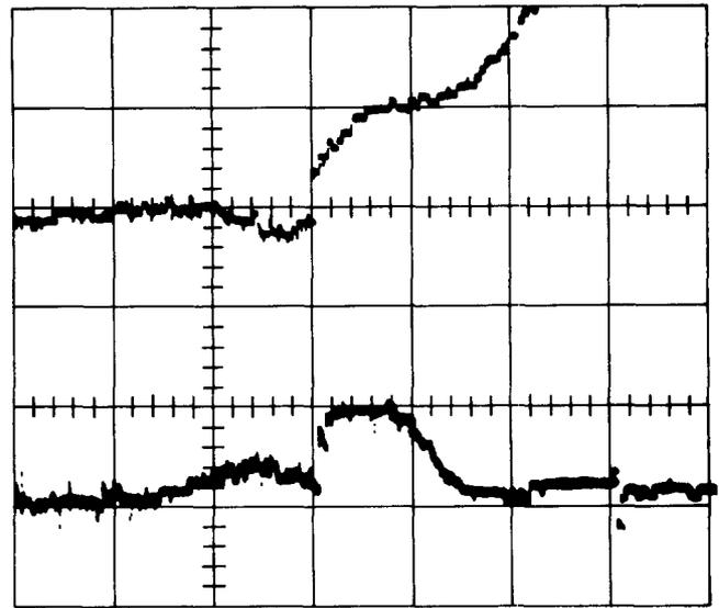
Fig. 5 Time dependence of voltage across test coil for pulses just greater and just smaller than the minimum quench energy. Vertical scale 1 mV/division, horizontal scale 1 ms/division, current 18 A
