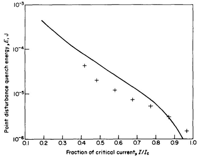
Fig. 3 Quench energy as a function of normalised current for a test coil at a constant field of 5 T. The solid line shows the calculated values and the crosses show experimental points
