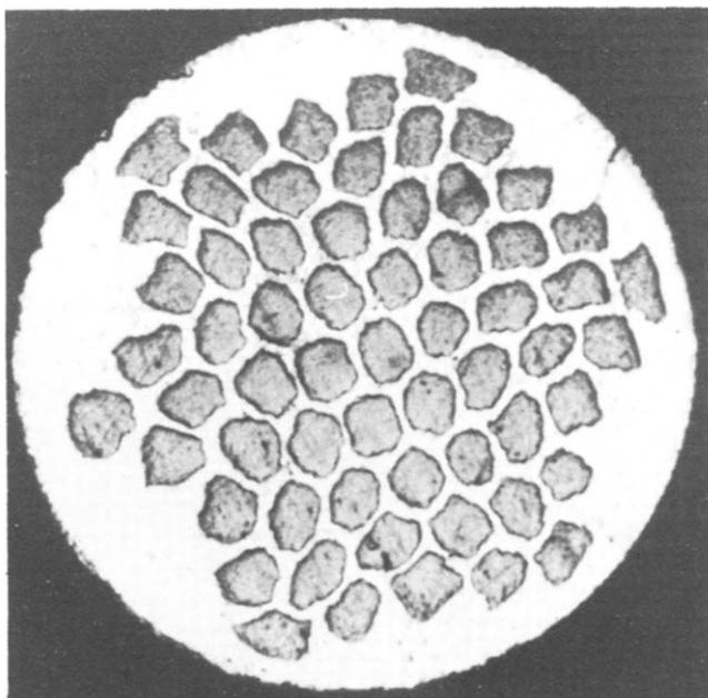
Fig. 4 Cross-section of superconducting composite, diameter 0.25 mm, IMI type A61/25 (copper matrix)
