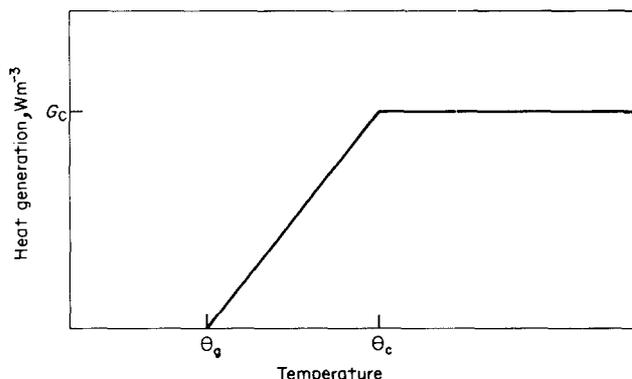
Fig. 1 Variation of heat generation with temperature at constant field and total current
